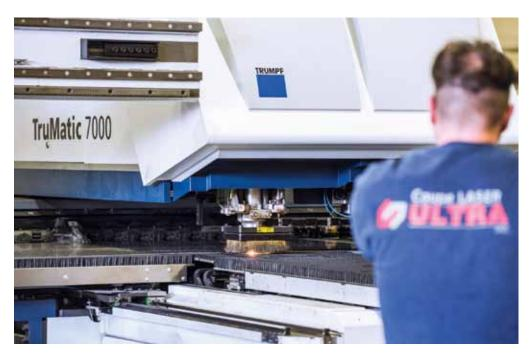
Able to hold 22 tools, the punch laser combo machine's punching head has a maximum stroke rate of 1,200 1/ min in the medium format (1,000 1/ min in large format).
